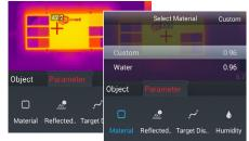
Select Material to change measured object's emissivity:
